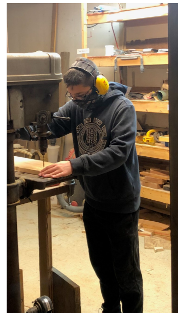
Brandon drilling holes for skateboard trucks
